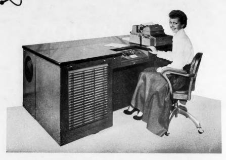
The MONROBOT is a general purpose digital computer, compact, ruggedized, reliable and reasonably priced. In the MONROBOT, decimal numbers are used. Since twenty digits are available, with a centrally located decimal point, there is no need for scaling or setting of decimal point. Neither overflow nor translation techniques are necessary. Orders are written for the calculator in virtually their original algebraic form.
